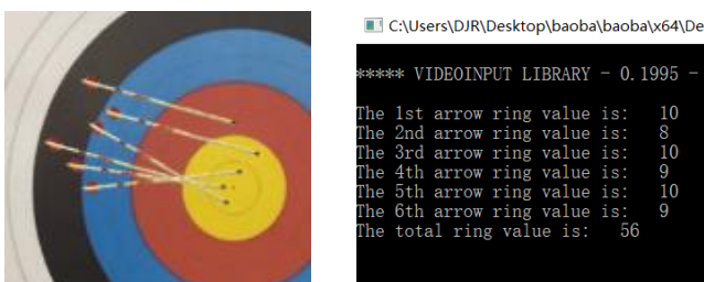
Fig. 19 Arrow tip occlusion test results
