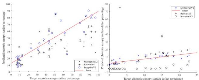
Fig. 7 Regression curves for deep transfer image regression approach of predicting necrotic and chlorotic surface defect percentages
