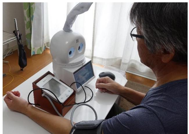
**Fig. 1** Frailty care robot AHOBO and its experimental scene in blood pressure measurement support situation.
