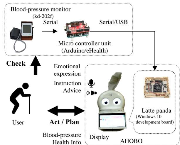
Fig. 6 Application for Blood-Pressure Measurement with AHOBO.
