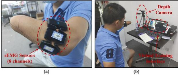
Fig. 1 System for sEMG and image recording. (a) sEMG system. (b) Depth camera and virtual training interface.
