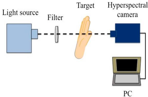
Fig. 7. Measurement system for transillumination imaging with hyper-spectral camera.
