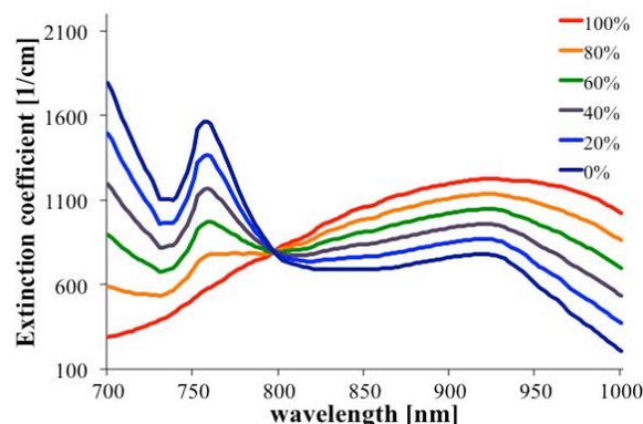
Fig. 6. Absorption spectra of Hb for different oxygen saturation.
