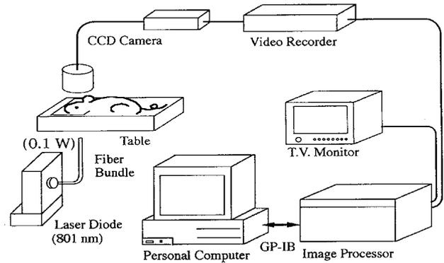
Fig. 1. System for transillumination imaging.
