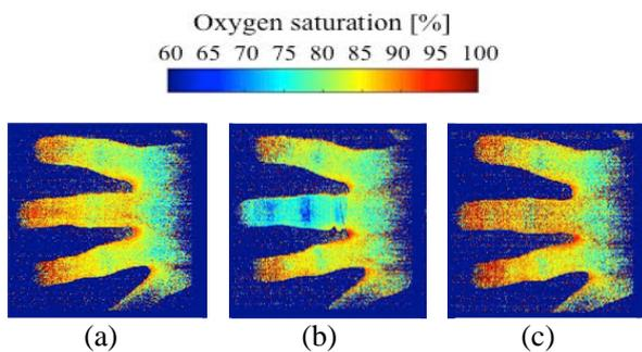
Fig.8. Temporal change of oxygen saturation in transillumination image in middle-finger constriction: (a) before constriction, (b) 11 minutes after constriction, (c) 11 minutes after release of constriction.
