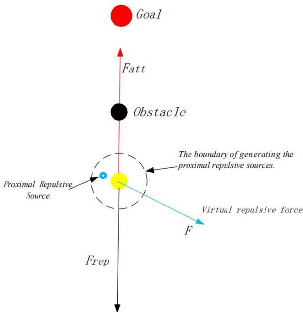
Fig. 3 Improved artificial potential field model
