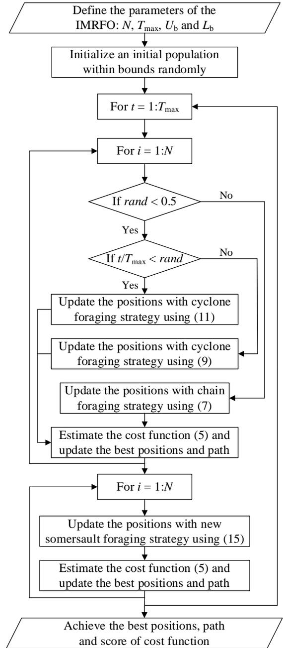
Fig. 2 Procedure of path planner based on IMRFO.
