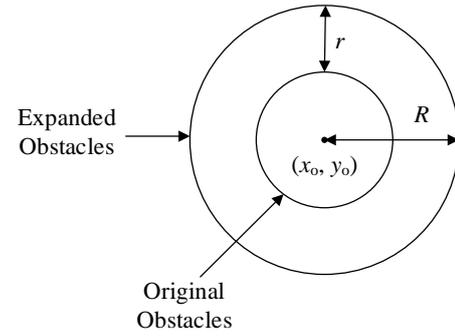
Fig. 1 Expanded obstacles size with mobile robot size.
