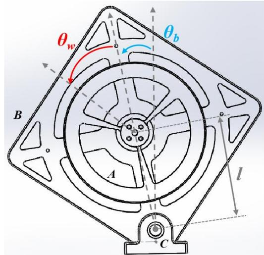
**Fig. 1** The schematic diagram of one-dimensional wheel pendulum model.
