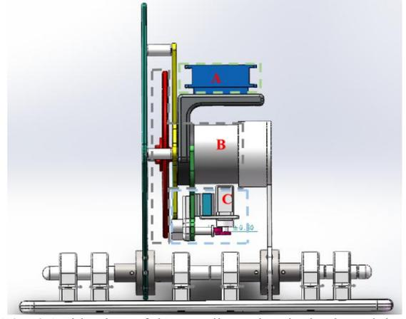
**Fig. 4** A side view of the one-dimensional wheel pendulum. The key modules in the system have been marked with dotted boxes: A. Control module, B. Drive module, C. Brake module.
