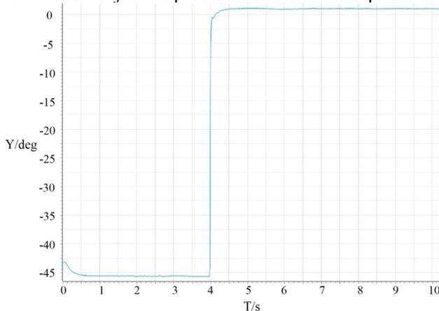
**Fig. 11** One-dimensional wheel pendulum model keep one-side balance after braking
