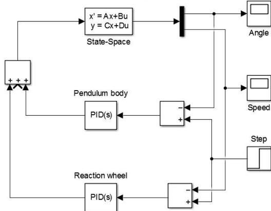
Fig. 5 The simulation Schematic of one-dimensional wheel pendulum model
