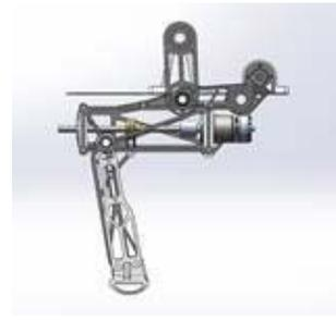
**Fig. 3.** Leg Structure Design
