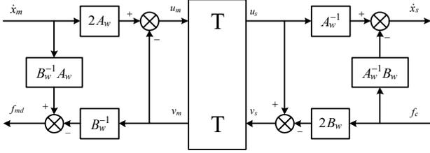
**Fig. 1** Wave variable structure
