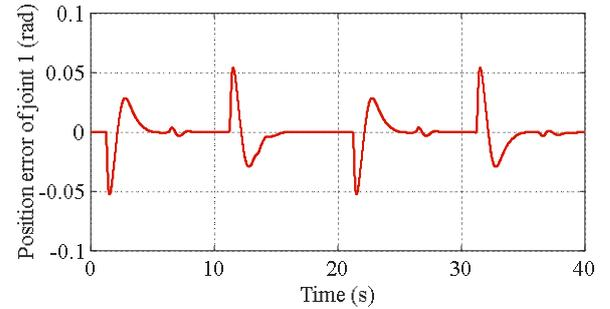
**Fig. 3** The joint tracking error between the master and slave
