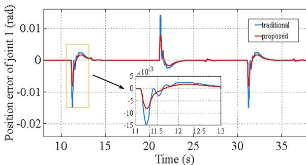
**Fig. 5** The comparison curve of the angle tracking error at the slave side
