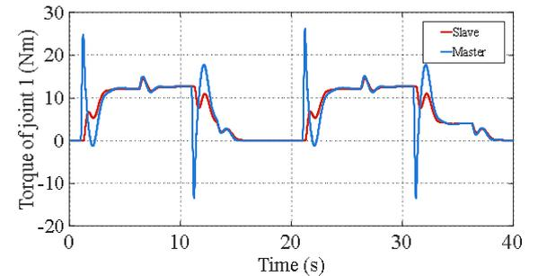
**Fig. 4** The torque tracking curve of the master and slave
