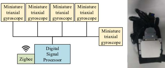
Fig.2. gesture measurement glove architecture
