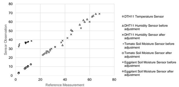
Figure 6: Calibration of Sensors using Reference Measuring Instruments
