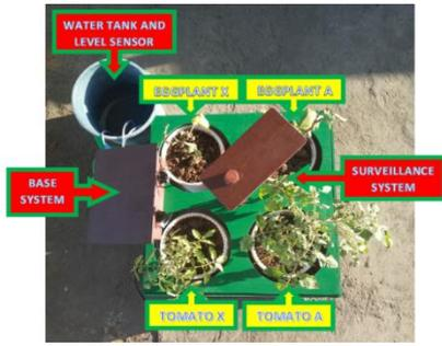
Figure 7: Deployment of the Irrigation, Monitoring and Control System
