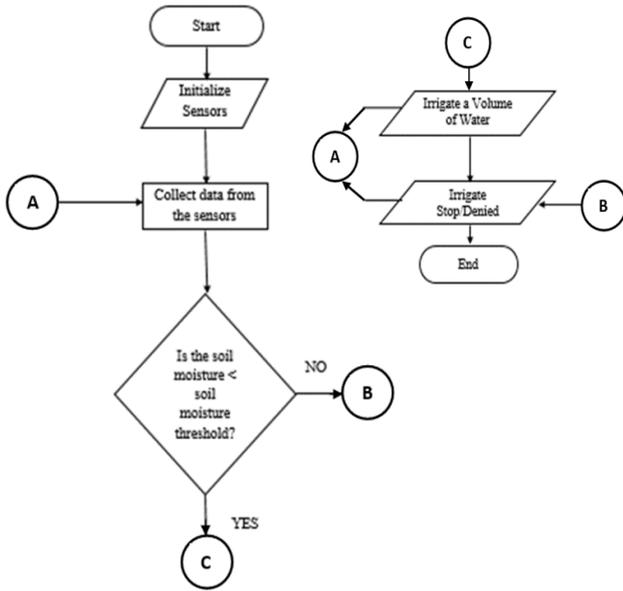
Figure 3: Precision Irrigation System Flowchart
