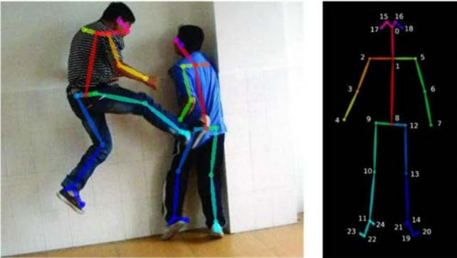
**Fig. 2.** Illustration of the campus violence skeleton-graph on the left. Illustration of the joints configuration by OpenPose on the right.
