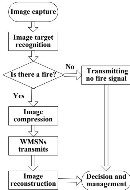
Fig.1. Fire detection strategy for wireless Multi-media sensor network
