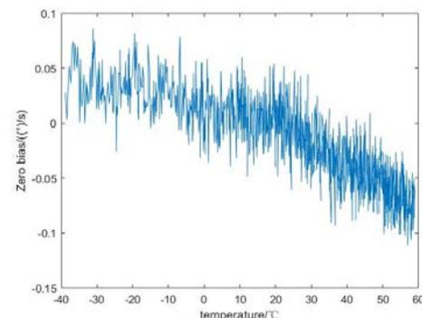
Fig. 3 Bias temperature relationship of new gyro samples
